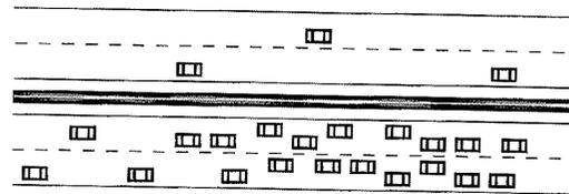
Figure 3. A traffic jam emerges from the behavior of all vehicles. New cars arrive as others leave, but the traffic jam remains. It can even move back while all cars are moving forward.
